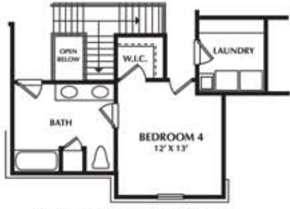
Opt. "F" LAUNDRY ROOM ON SECOND FLOOR TO BE BUILT IN CONJUNCTION WITH OPTIONS D & E
